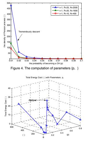
Figure 5. Optimal value p for minimizing total energy cost  $(\delta)$
